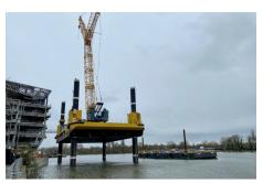
**EuroJack-ups: stable jack-up platforms for civil construction and offshore operations.** Our versatile EuroJack-up barges provide stable platforms for maritime construction and other missions both near and offshore.
