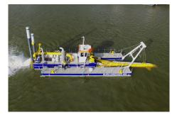
EuroCutters: powerful and essential tool in many dredging and marine operations. Cutter suction dredgers are specifically designed to dredge compact and hard soils under the waterline.
