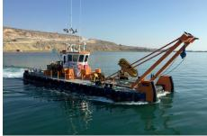
Modular Pontoon Systems (MPS): modular pontoons, jack-ups and workboats. Neptune offers Modular Pontoon Systems (MPS) for the on-site assembly of pontoons and workboats in areas of restricted access.
